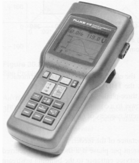
Figure 30.45 This portable instrument, the “Power Harmonics Analyzer” can measure the total harmonic distortion (THD) of a voltage or current up to the 31 st harmonic. It can also measure the active, reactive and apparent power in a 3-phase circuit, and its power factor. It also gives a readout of the K factor of a current (courtesy of Fluke Electronics Canada Inc.).
